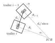
Finally, the kinematic model of a car pulling  ${\cal N}$  trailers can be written as
