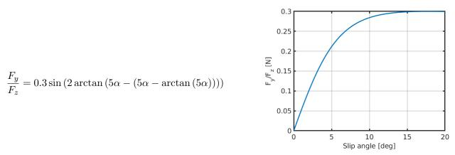
Determine, using the Magic Formula and motivating the result, the value of the cornering stiffness, and draw on the picture the cornering stiffness approximation of the lateral force/slip relation.
