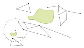
where the black dots are the nodes sampled in previous iterations, the red dot is the node sampled in the actual iteration, the green blobs are obstacles and the black dashed circle is the neighbourhood considered to defined the Near set.
