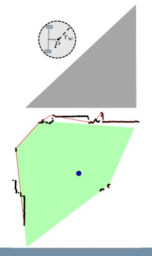
Once the allowed admissible convex state region has been determined, it can be represented as a set of linear constraints  $h_1^j x_P (k+i) + h_2^j y_P (k+i) \le l^j \qquad j = 1, \dots, n_c$
