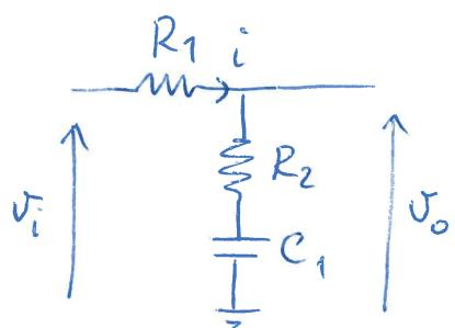
$$C_1 \frac{dV_C}{dt} = i = \frac{V_i - V_o}{R_1}$$
