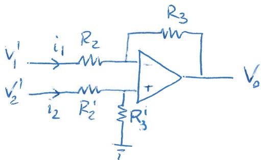
$$i_1 = \frac{V_1' - V_o}{R_2 + R_3}$$
