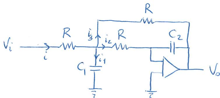
$$\begin{cases} R i_3 = R i_2 + V_{C_2} = R i_2 - V_o \\ i_2 = C_2 \frac{dV_{C_2}}{dt} = -C_2 \frac{dV_o}{dt} \end{cases} \Rightarrow i_3 = -C_2 \frac{dV_o}{dt} - \frac{1}{R} V_o$$
