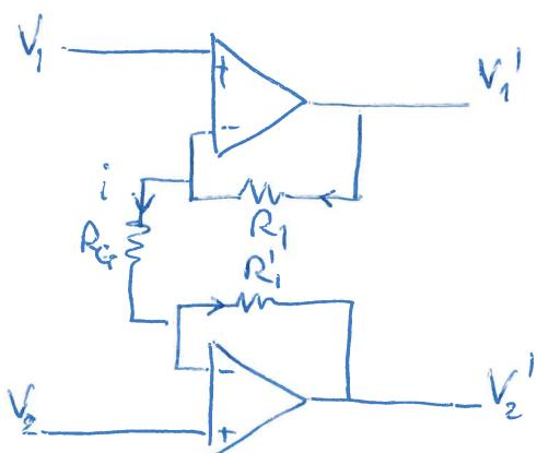
$$i = \frac{V_1 - V_2}{R_G}$$
