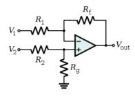
**6.2** Determine the values of the resistors so that the previous circuit acts as a differential amplifier with gain equal to 10.
