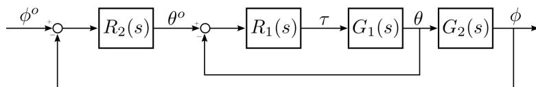
3. Compute a digital realization of the controllers designed in the previous steps, and simulate the digital control system assuming that the analogue to digital converter is characterised by 12 bit over a range of  $360^\circ$ , and the digital to analogue converter is characterised by 14 bit over a range of  $\pm 5 Nm$ . Simulate the response of the system to a ramp with slope  $0.1 rad/s$ .
