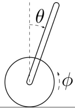
where  $\phi$  and  $\theta$  are the angular position of the wheel and the rod, respectively,  $\tau$  is the motor torque, and
