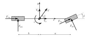
write the Newton equations of the translational motion of the center of mass of the bicycle, and the Euler equation of the rotational motion, both referred to the body frame.
