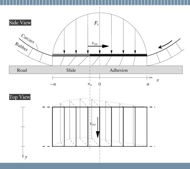
We assume that static and kinetic (sliding) friction coefficients are equal, the force acting on brushes during sliding is thus  $\mu F_{zi}$ .
