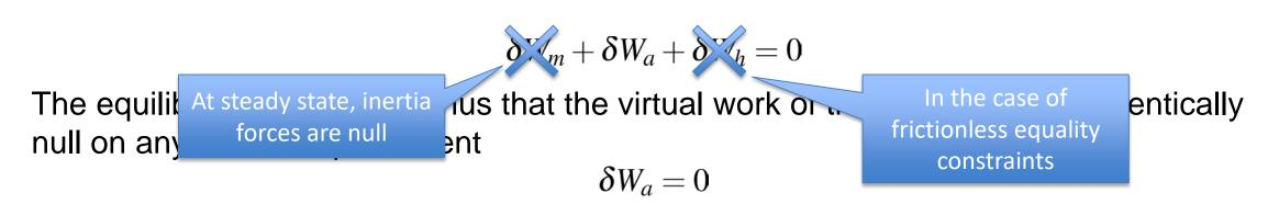
This is known as the *principle of virtual work* and is the fundamental equation of statics of a constrained system.
