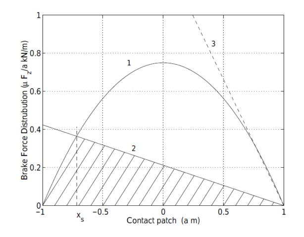
Recall the relation we use to compute  $x_s$   $c_p \sigma_x (a - x_s) = \mu q_z (x_s)$ If slip increases the magnitude of the slope  $c_p \sigma_x$  increases.
