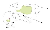
where the black dots are the nodes sampled in previous iterations, the red dot is the node sampled in the actual iteration, the green blobs are obstacles and the black dashed circle is the neighbourhood considered to defined the Near set.
