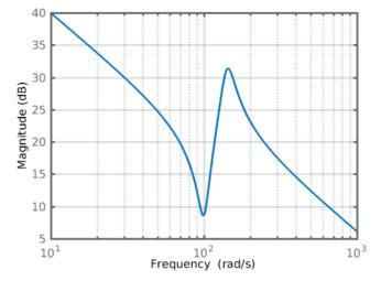
**5.2** Design a PI velocity controller, accurately describing the procedure, that maximizes the damping of the oscillations generated by the elastic transmission.
