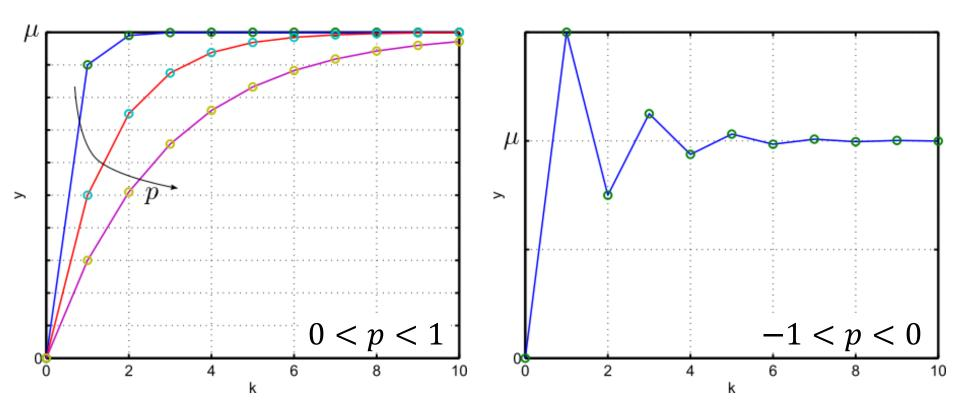
A peculiarity of discrete time systems: even the step response of a first order system can exhibit oscillations.
